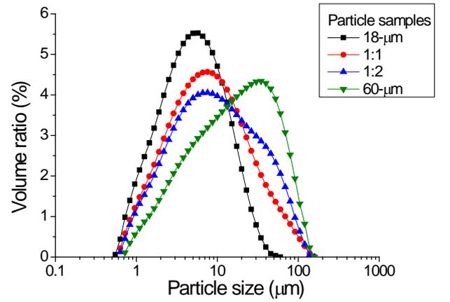
Figure 2. Particle size distributions of the silica samples.
