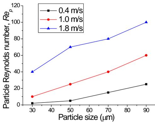
Figure 4. Simulation results of  $Re_p$  for three inlet velocities [20].
