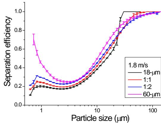
Figure 5. Separation efficiency curves with their standard deviations for four particle samples at the inlet velocity of 1.8 m/s.
