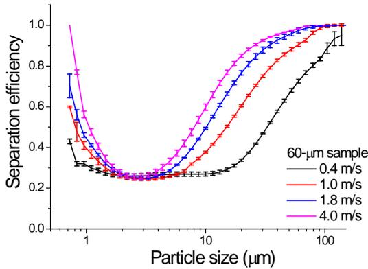
Figure 3. Separation efficiency curves with their standard deviations for four inlet velocities.
